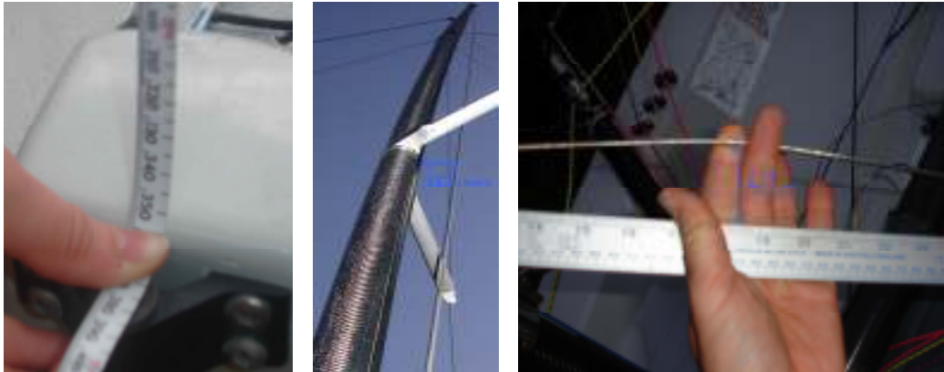
Figures measuring from left to right rake, pre-bend and lowers deflection.
