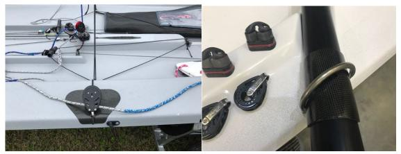
• The holes through the gunwales that take the trapeze elastic and the elastic away from the front of the wing tubes will have neat little bushes fitted, as per the Aero. It will save on wear and look neater. (see picture 4)
